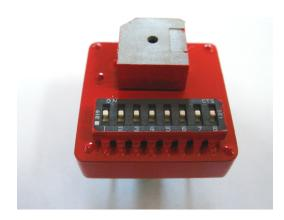
This is a microprocessor controlled engine cooling system for the DeLorean engine. Program switches can be user selected to select cooling fan operation for user preferred operation.
