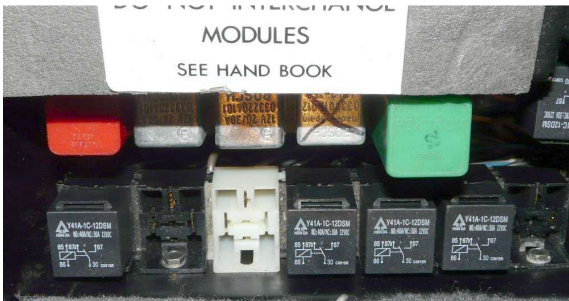
Figure 2. White relay socket and relay bank mounting screws.
